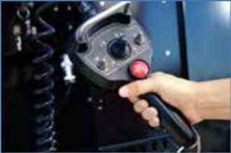
2 Proven tethered ground drive controller allows you to maneuver the drilling unit to a position that provides better visibility, easier loading/unloading and easier positioning.
