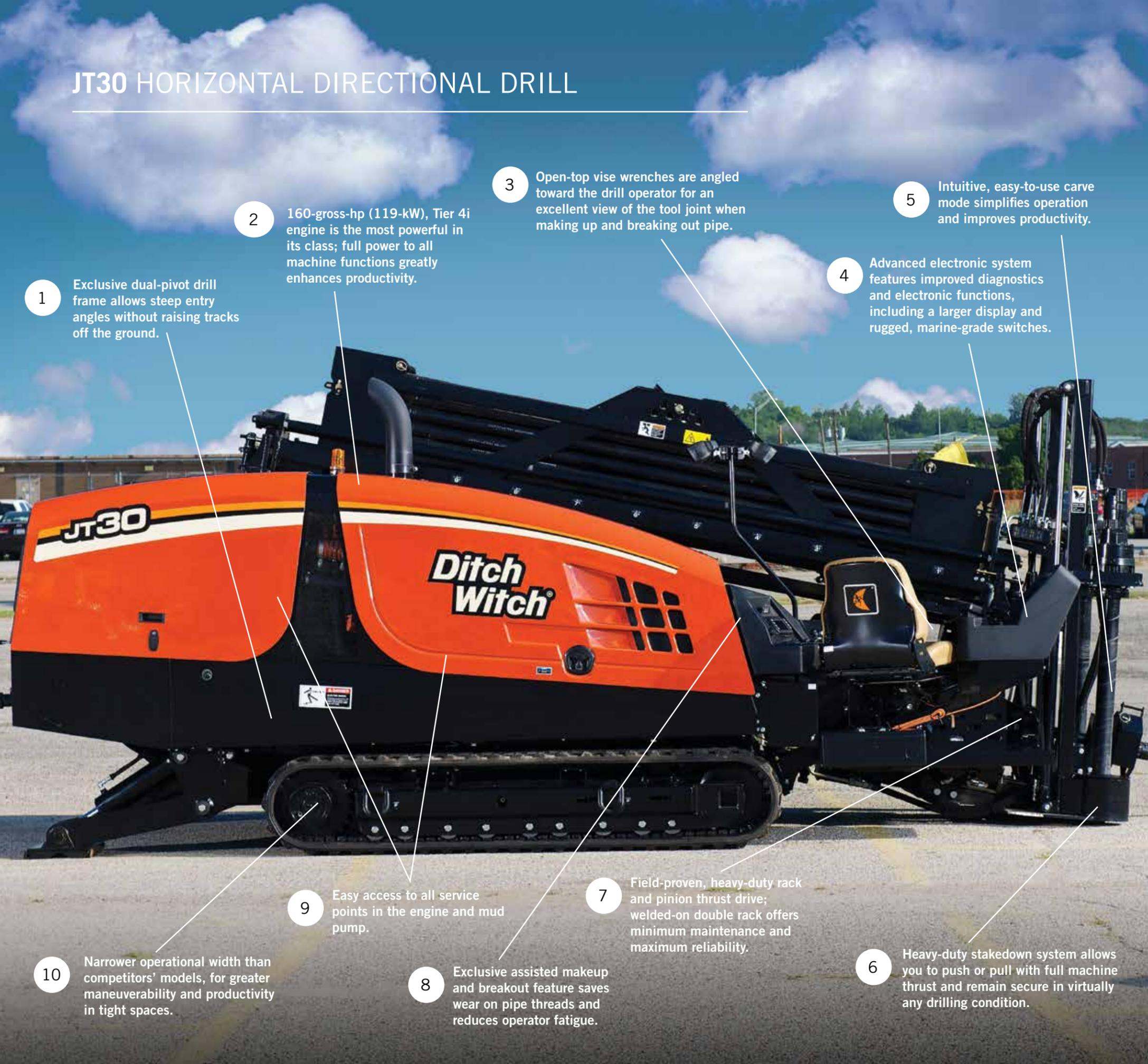
1 Exclusive dual-pivot drill frame allows steep entry angles without raising tracks off the ground.
