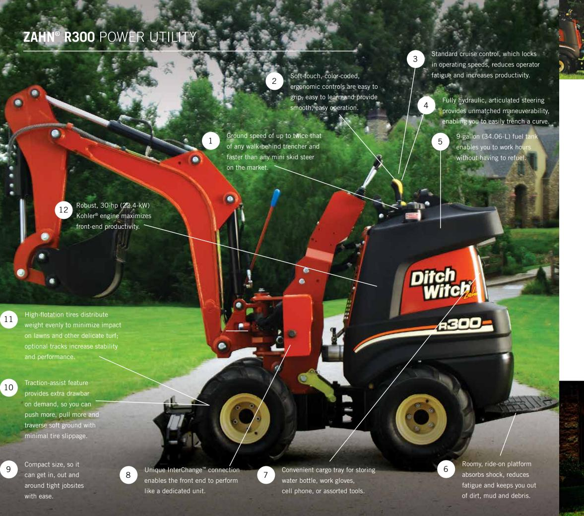
The Ditch Witch® Zahn® R300 is the best compact trencher ever made—and also the best backhoe, tool carrier and vibratory plow. With an ordinary machine with attachments, you expect to give up a little performance. But the Zahn R300 is nowhere near ordinary. With its unique InterChange™ connection, the front end becomes the machine and performs like a dedicated unit. With the Zahn R300 you get more power, more speed and, best of all, more productivity.
